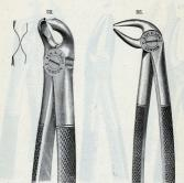
Fig. 32 for lower Molars with decayed and broken down crowns. The points on the beaks go between the two roots and relieve the pressure which there would otherwise be on the frail walls that may remain. Made with straight handles, beaks finely serrated inside and adapted for use on either side of the mouth.
