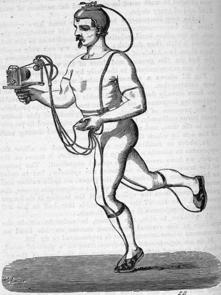
FIG. 27.—Runner provided with the apparatus intended to register his , different paces.
