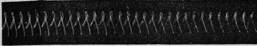
FIG. 79.—Tracings of a Wheatstone rod tuned to the octave, furnished with the wing of a wasp, and arranged so as to register especially the upper loop of the 8.
