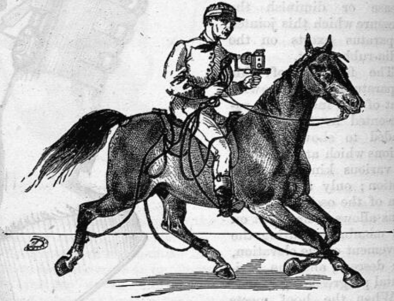
FIG. 44.—This figure represents a trotting horse, furnished with the different experimental instruments; the horseman carrying the register of the pace. On the withers and the croup are instruments to show the reactions.
