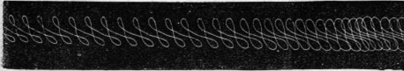
FIG. 76.—Tracing of a Wheatstone's kaleidophone rod, tuned to the octave, that is to say, vibrating twice transversely for each longitudinal vibration. (This figure is taken from R. Koenig.) The slackening speed of the cylinder produces an approximation of the curves towards the end of the figure.
