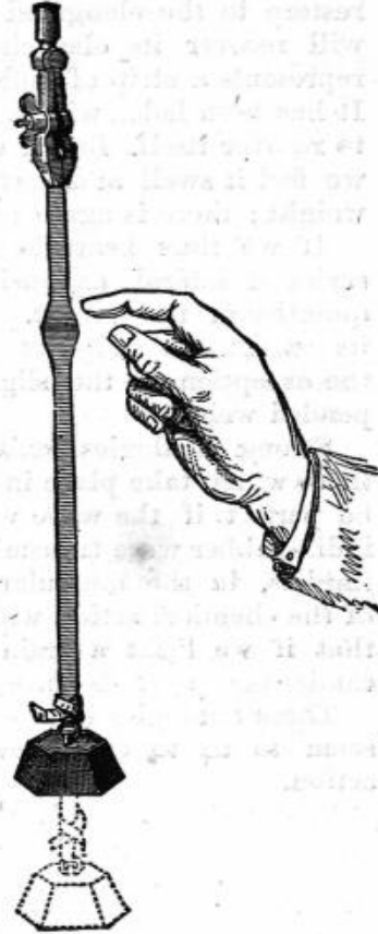
FIG. 9.—Transformation of heat into work by a strip of india-rubber.
