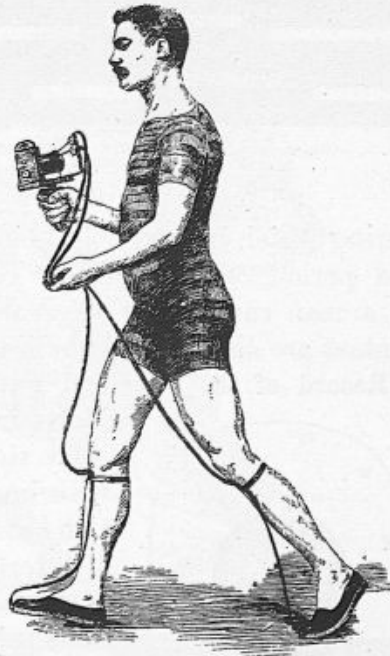
FIG. 4.—Pedestrian furnished with special shoes and carrying a chronographic apparatus.
