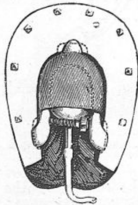
FIG. 6.—Special apparatus for recording the contacts of a horse's feet with the ground; a transmitting tube effects a communication between the air chamber and the chronographic tambour.
