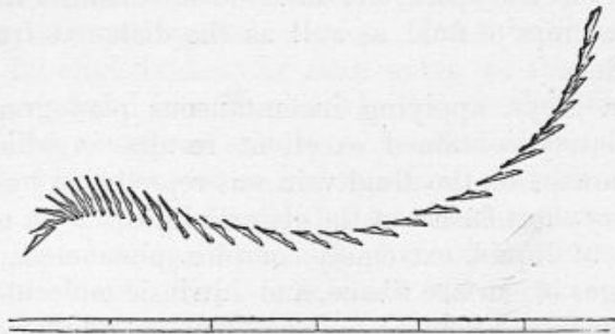
FIG. 59.—Chronophotographic trajectory of a flying apparatus describing a sinuous curve in the air (20 images to the second).
